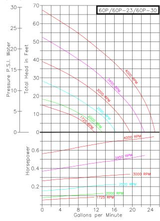
The flow produced is not positive which permits the discharge line to be shut off completely without danger of overloading motors or bursting lines. Consequently a relief valve is not required.
